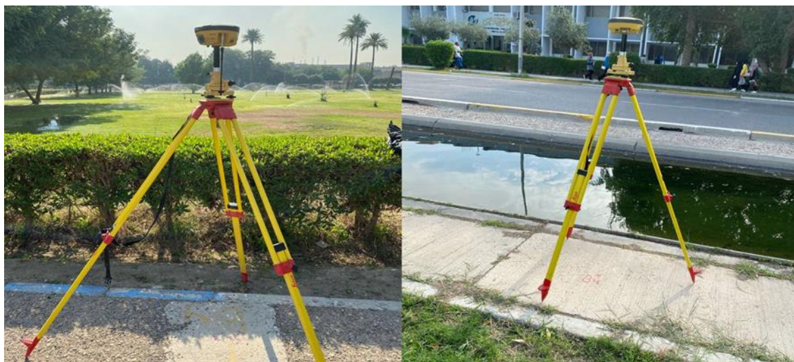
Figure 3: Collecting Ground Control Point Using DGPS
