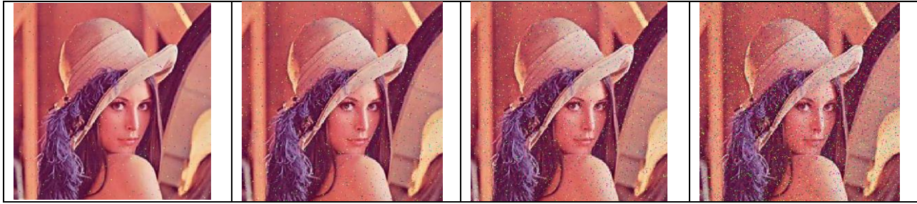
Figure 5 illustrates the impact of noise attacks on an encrypted image. Panel (a) shows the encrypted image with a low level of salt and pepper noise (0.01), while panels (b), (c), and (d) display the image with progressively higher noise levels (0.03, 0.05, and 0.1, respectively).
